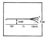
Tapes recorded on one deck can be played back on another. However, slight differences occur between any two decks such as playback frequency response and head azimuth. This occurrence is noticeable when using the Dolby NR system. To solve this problem, this unit incorporates a newlydesigned PLAY TRIM control.
